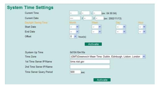
The PT-7728 has a time calibration function based on information from an NTP server or user specified time and date. Functions such as automatic warning emails can therefore include time and date stamp.
